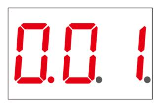
DMX signal indicator : When DMX signal input is detected, the indicator on the display following after the digit of "hundreds" position of DMX address turns on red . If there is no signal input, the dot indicator will not turn on, and the "hundreds" position of DMX address will flash.
