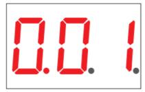
**DMX signal indicator** : When DMX signal input is detected, the indicator on the display following after the digit
