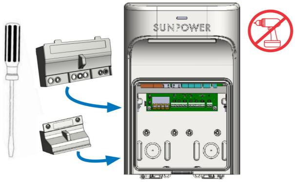
**Warning!** To protect against the risk of electrical shock reinstall the AC wiring covers before reenergizing the equipment.
