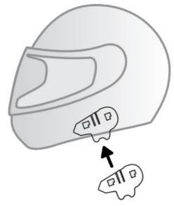
3. Align the clamping position of the main unit base at the clamp fastener, and move the main unit at the direction of Arrow 1 first followed by the direction of Arrow 2 to tighten it.
