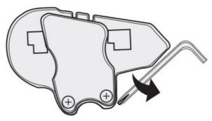
2. Open the inner lining on the left of the helmet to mount the clamp at a proper position and then tighten the screws.
