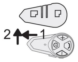
2. Peel off sticker on back of velcro clip and stick it in place on left side of helmet.
