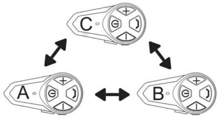
Note: Clear the pairing record of each machine before pairing.
