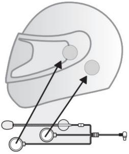
6. Attach circular microphone rod to a suitable position on left side of helmet, so that microphone is aimed at mouth, and then adjust line and inner linings.
