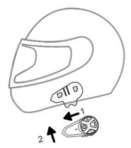
4. Open inner lining at ear position of helmet and attach velcro surface on speaker of the headphone cable.
