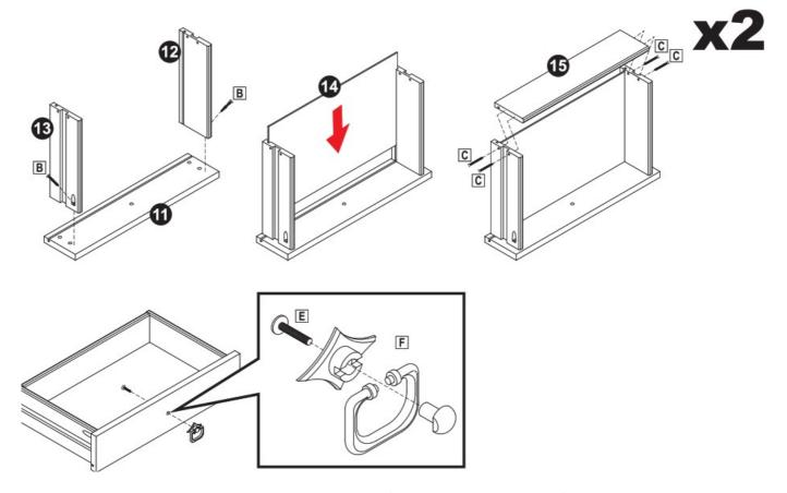
Ensuring the inside grooves align, secure Right Drawer Side (12) and Left Drawer Side (13) to Drawer Face (11) using two M4.5x28mm Pan Screws (B).
