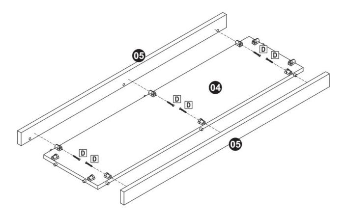
Align two Shelf Aprons (05) with Shelf (04) and secure using six M4.5x25mm Pan Screws (D).
