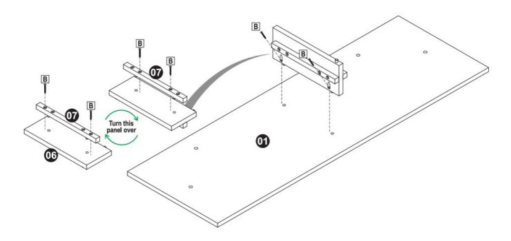
Align one Inside Drawer Rail (07) with Center Panel (06) and secure using two M4.5x28mm Pan Screws (B). Flip the panel over and repeat to secure the remaining inside drawer rail.
