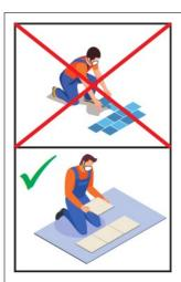
Assemble on a soft, flat, clean, and dry surface.
