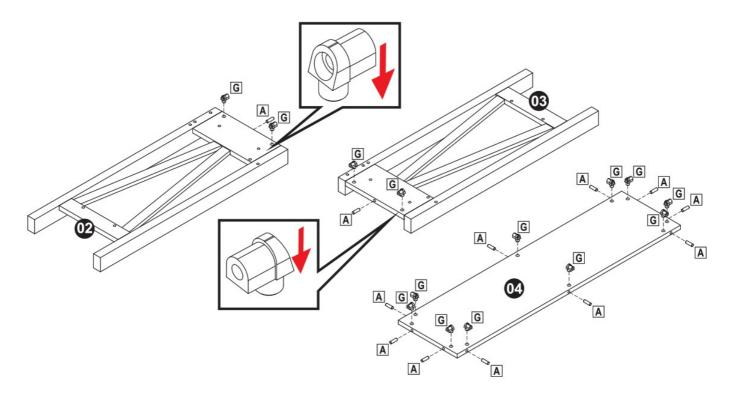
Install one Wood Dowl (A) into Right Side Panel (02) and Left Side Panel (03), as shown.
