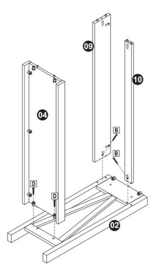
Secure Back Panel (09) to Right Side Panel (02) using one M4.5mmx28mm Pan Screw (B). Then, secure Front Crossbar (10) using one M4.5mmx28mm Pan Screw (B). Secure the shelf using two M4.5x25mm Pan Screws (D).
