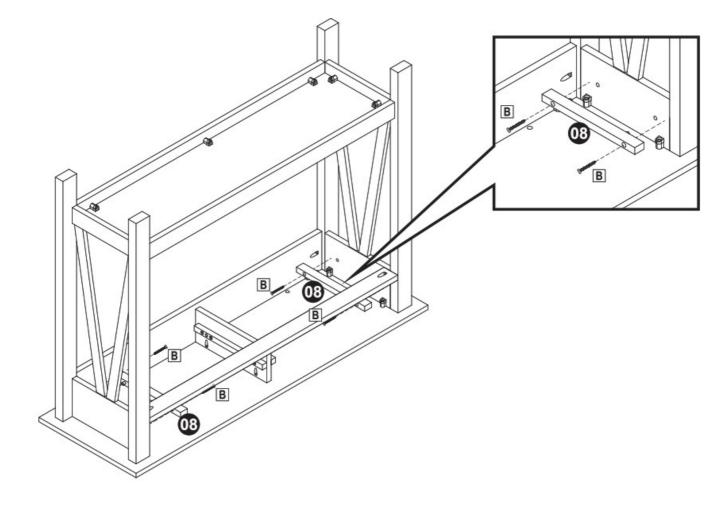
Align one Outside Drawer Rail (08) with one of the side panels and secure using two M4.5x28mm Pan Screws (B). Repeat to secure the remaining outside drawer rail to the opposite side panel.
