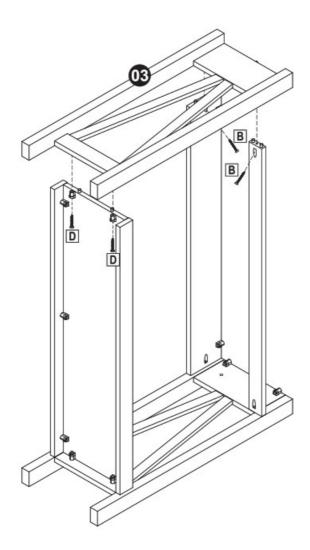
Secure Left Side Panel (03) using two M4.5mmx28mm Pan Screw (B) and two M4.5x25mm Pan Screws (D), as shown.
