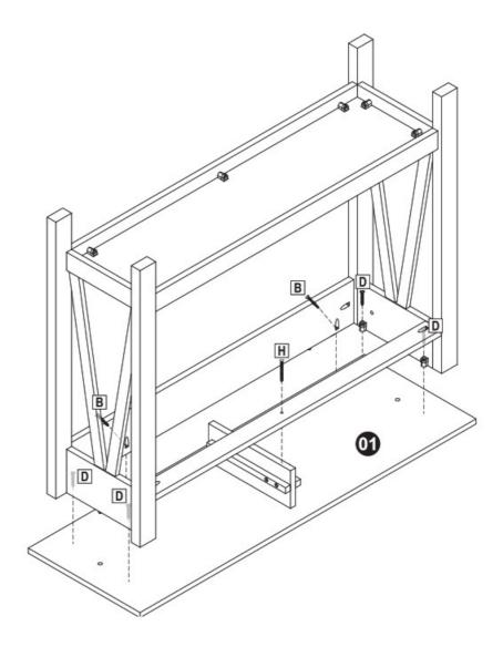
Align the assembled frame with the top.
