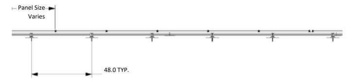
48" is typical span between attachments for many areas. Check local code for span requirements.
