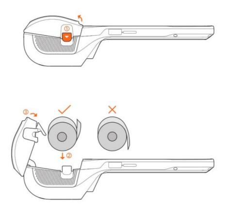
This device can load a 80mm thermal receipt or label paper roll, and black label is also optional.
