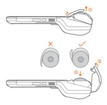
This device can load a 58mm thermal receipt or label paper roll.
