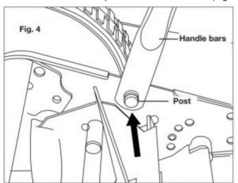
5. Pull both sides of the lower handle bars over the posts on the mower body. Press inward on the handle bars to
