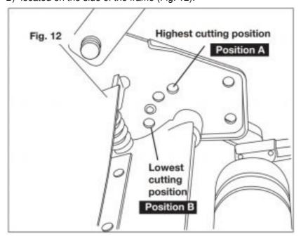
5. Other cutting heights are achieved by moving the adjustment knobs to the settings between the highest and lowest positions.
