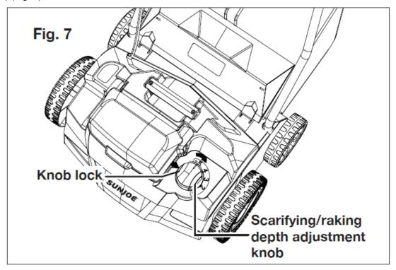
2. This scarifier + dethatcher is equipped with 5 scarifying/raking depths. When assembled with different cylinder, each setting indicates different depth. Check the table below for details about each setting.
