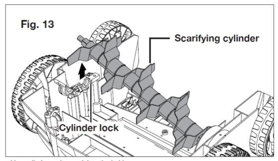
4. Insert the raking cylinder and press it into the holder.
