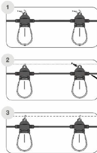
1. Temporary mounting: Using standard S hooks (not included) or screw hooks (not included) the solar string lights can be mounted utilizing the integrated mounting loops.
