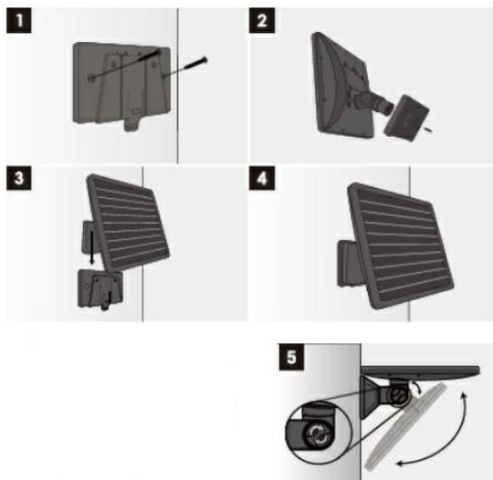
1. If required use the two wall plugs (H) along with the two large screws (G). Install the screws utilizing the two outer holes of the mounting bracket to secure the bracket to the chosen surface.
