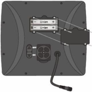
The solar string light's batteries (I) are installed on the rear of the solar panel. Always open the battery compartment with the ON/OFF switch in the OFF position. Unscrew the back of the battery compartment and remove the backing piece. Inside you will see the batteries. When replacing the batteries, observe the correct polarity and match the battery specifications with the batteries you have removed.
