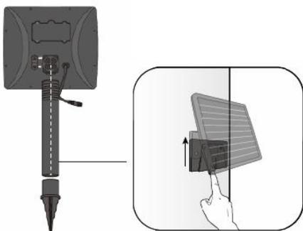
**Note:** To disconnect the solar panel from the mounting bracket, press down on the release tab on the bottom of the mounting bracket. With the tab firmly pressed, slide the solar panel upwards and free of the bracket. Some force may be required to remove the panel from the bracket.
