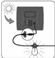
1. Connect the solar panel to the connector on the string lights.
