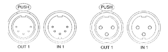
XLR 5-pin connectors are used to connect external master and slave devices to DMX ports. If necessary, the device can be equipped with XLR three-pin connectors. Each port on the 2 and 4-port devices has 2 connectors one M connector and one F connector, which allow the port to pass-through the DMX bus. On 8 and 16 port devices and ArtGate Compact, each port has single connector of type F. Each port is equipped with internal 120 ohms terminator which can be enabled via web interface.
