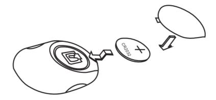
Positive pole upwards to install the battery.
