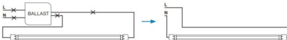
Wiring Diagram B: Shunted Double-Ended Wiring
