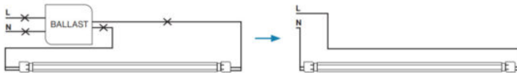
Wiring Diagram A: Non-Shunted Double-Ended Wiring
