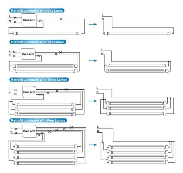
**Non-Shunted Double-Ended Wiring Diagram**
