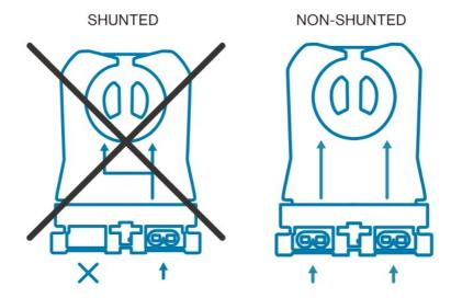
Double-Ended: Non-Shunted and Shunted Compatible
