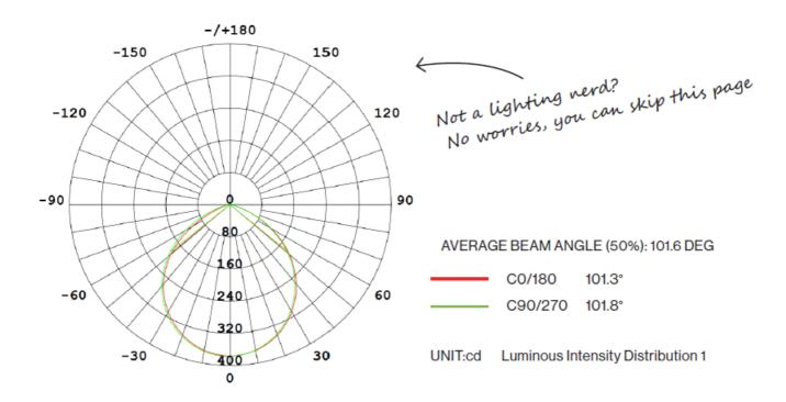
Lighting distribution angle refers to the spread of light emitted from a light source. It is an important factor to consider when selecting a fixture or bulb, as it affects the way it will illuminate an area. There are two main types
