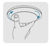
**Step 1**Remove the lens by twisting clockwise.
