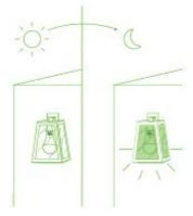
Sunco D2D lights turn on/off automatically and do not require a timer to activate. Avoid using them with a timer on the same circuit.
