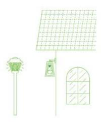
If a Dusk to Dawn LED is installed too close to another switched on light, the sensor may be fooled into thinking the light detected is daylight.
