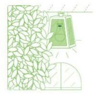
Even an open light fixture cannot function when hidden behind a tree or shrub. Here, the light is on during the day, because sunlight is not reaching it.
