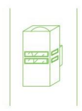
The Dusk to Dawn sensor cannot detect whether it is light or dark when the light fixture is closed.
