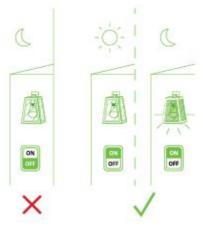
At night, the left D2D LED cannot turn on as there is no power. In contrast, the D2D on the right has power and the sensor can function properly.
