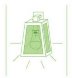
In an open fixture, the sensor will detect light through the clear glass panes and turn on at night.
