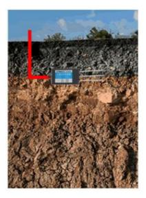
Dig a pit with a diameter of about 20cm vertically, and insert the steel needle of the sensor into the pit horizontally according to the measurement needs, compact the soil in the pit to ensure close contact with the soil. After the sensor is stable for a period of time, continuous long-term measurement and recording
