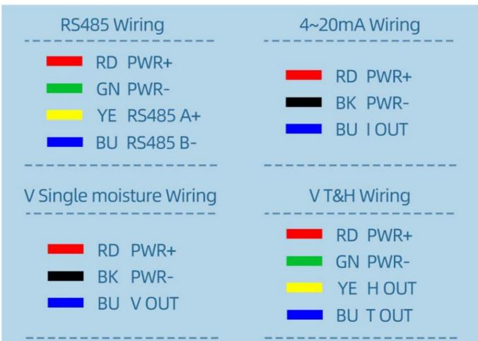
**Note:** When wiring, first connect the positive and negative poles of the power supply, and then connect the signal line
