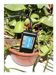
measurement, maintain the original tightness of the underlying soil, hold the sensor vertically into the soil, and do not shake it left and right when inserting to ensure close contact with the soil
