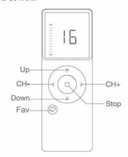
• Wall-Mounted 16-channel LCD Remote Controller
