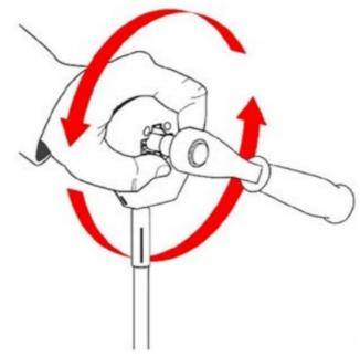
• To re-lock the booster and shade, release the wand control and rotate the Socket Ratchet enough to re-engage the lock (approx. 1/4 turn). The ratchet should spring back under the spring tension to the locked position.
