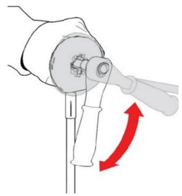
• Hold the shade and Wand Control Head together. To add tension, rotate the Socket Ratchet for the number of turns desired in a counter clockwise. (Note, to remove tension allow the spring to unwind in the clockwise
