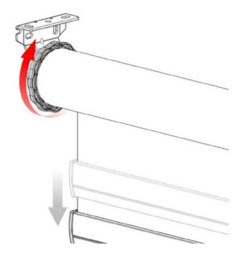
To raise the top limit position rotate the limiter head so that the Shade rises.
