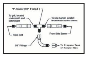
You will need a 'T' adapter fitting (not provided) or a similar connection to connect a single gas line to both a side burner and a grill. We recommend a licensed gas technician install all gas lines. See the below figure for the installation of a 'T' adapter.
