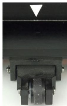
Defective pinch roller Out of center
