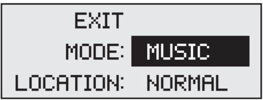
Rotate the MASTER knob to scroll through the menu items. When the desired item is highlighted, press the MASTER knob to select it. The parameter value that you will be adjusting will be highlighted.
