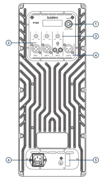
A fuse is included within the IEC socket for added protection – if the fuse fails ensure it is replaced with a fuse of the same type and rating.
