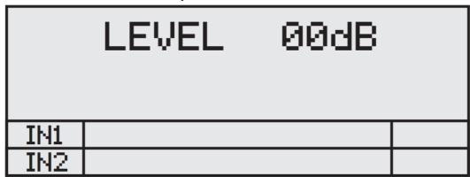
The signal levels for each of the two input channels are shown as a horizontal bar graph. `CLIP' appears in the box at the right-hand side of the graph if the input signal level exceeds the clipping level. Reduce the input level if this happens.
