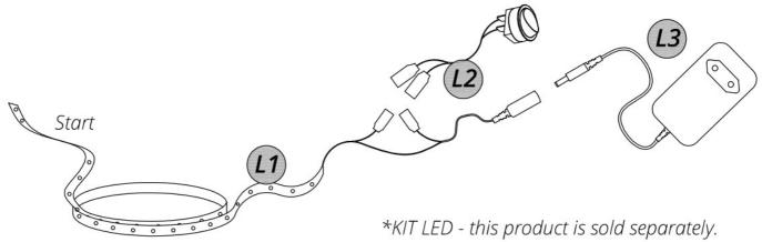
Remove the protective film from the double-sided tape and start gluing the LED tape on the side of part n° 06 in the position indicated by the arrow. Go pasting the tape by pieces n° 06, n° 07, n° 06 and finish gluing at the end of piece n° 07.
