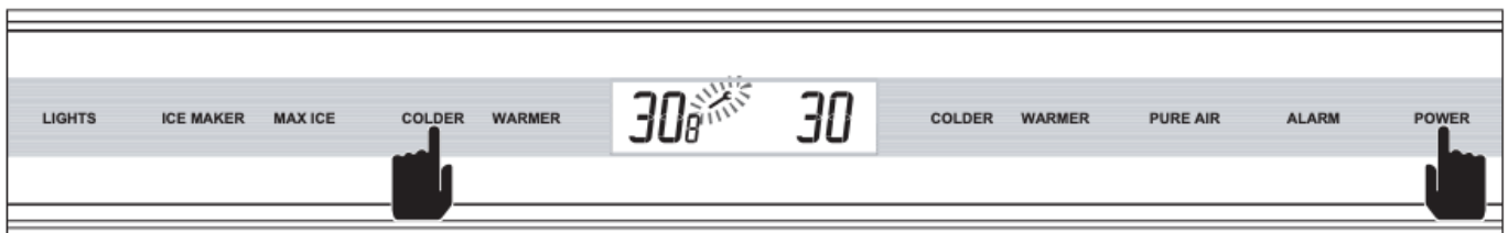
Figure 7-3. Initiate Fault Code Mode - Press and Hold a COLDER Key, Then the POWER Key
