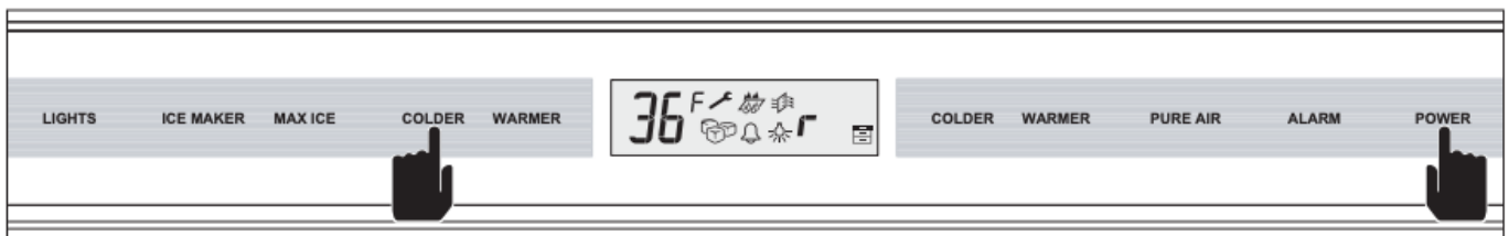
Figure 7-1. Initiate Diagnostic Mode - Press and Hold a COLDER Key, Then the POWER Key
