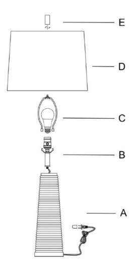
Use 100 watt or smaller type A bulb (not included) or use maximum 9 watt LED bulb (included).
