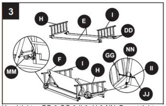
Hand tighten DD & GG & II & JJ & NN. Do not tighten with wrench, OO & PP until all bolts have been installe d.
