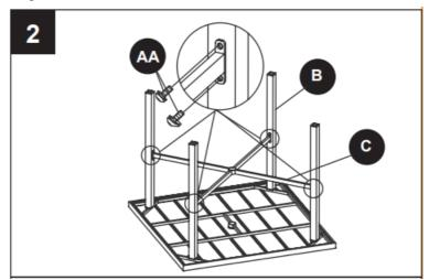
2. Hand tightens AA. Do not tighten with a wrench, or BB, until all bolts have been installed.
