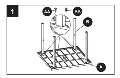
1. Hand tightens AA. Do not tighten with a wrench, or BB, until all bolts have been installed.
