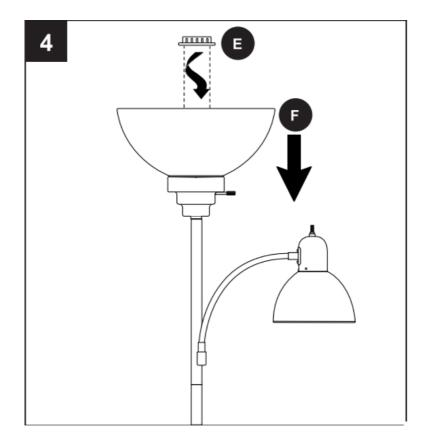
Do not overtighten (E) as (F) may crack or break.
