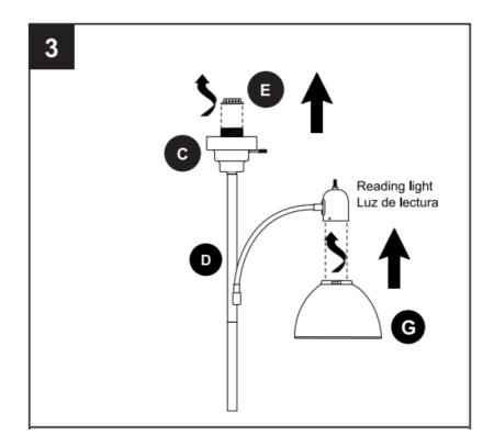
Align grooves on (G) with nodules on inside reading light and push up gently on (G). Turn (G) to the RIGHT (clockwise) until (G) slides completely into place.
