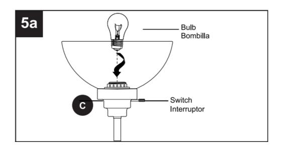
Use a 40-watt max. incandescent bulb (not included) or CFL/LE equivalent.
