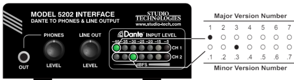
Figure 2. Detail of the front panel showing the LEDs that display the firmware version. In this example, the version
