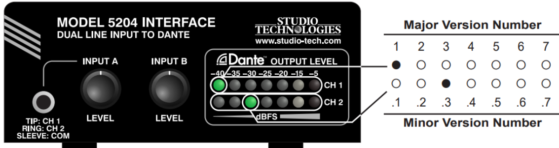
Figure 2. Detail of front panel showing the LEDs that display the firmware version. In this example, the version shown is 1.3.
