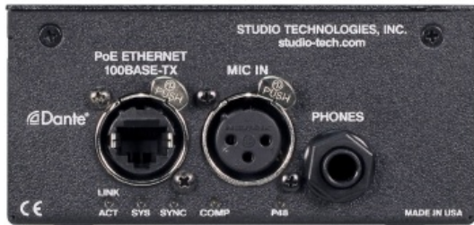
Figure 1. Model 203 Announcer's Console front and rear views
