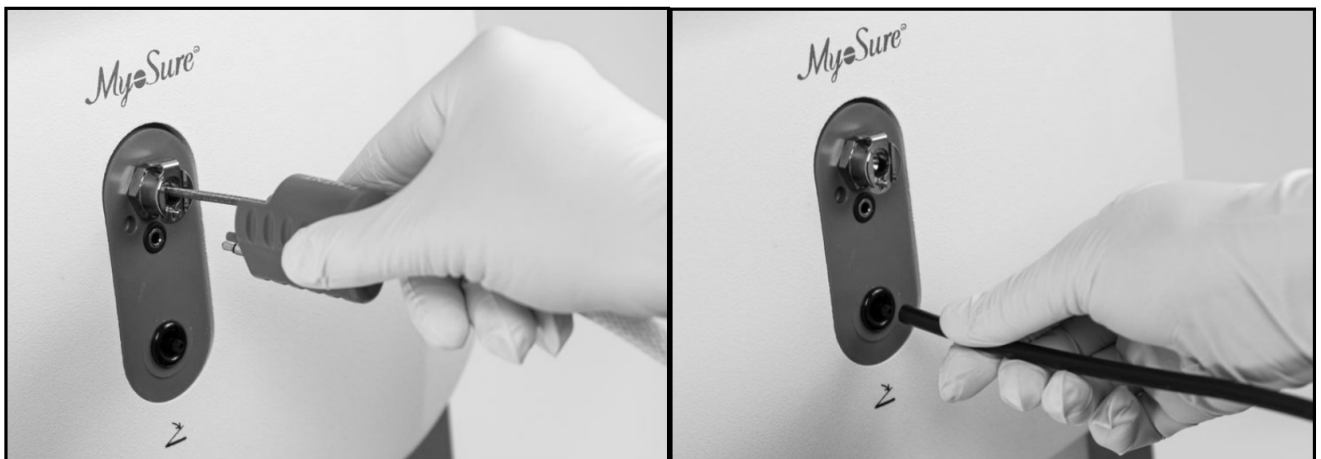
FIGURE 3: INSERT DRIVE CABLE AND FOOT PEDAL INTO FLUENT FLUID MANAGEMENT SYSTEM
