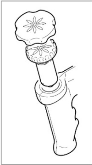
Figure 6: Cryogen canister removal and/or replacement
