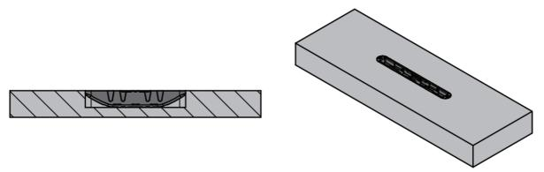
6. The Mini 60 features locating tabs which click into place when fully assembled. Please note this feature is not a lock, making the joint fully reversible.
