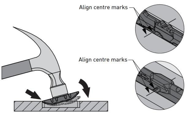
5. After glue is applied, insert Key and Hook into slot until flush with substrate. Allow to dry as per glue manufactures instructions.
