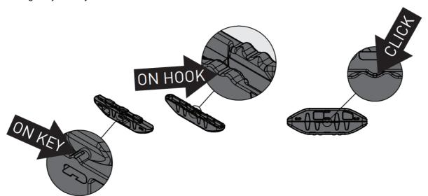
7. Assembly components remembering the Key only needs to travel 1 pitch for full engagement. This is detailed in steps A and B.
