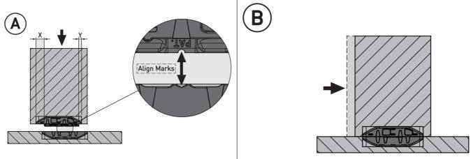
Note the offset of the lugs on the Key body, length X is larger than Y. Insert the Hook into the Key with the lon ger X end towards the face to be pushed during assembly.
