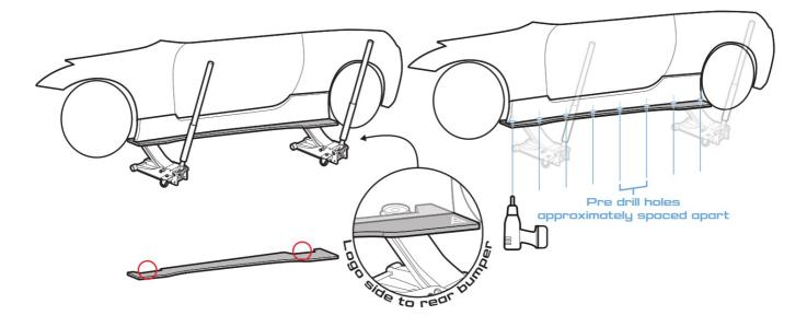
**NOTE:** Position the jack stand at the Side Splitter's pinch welds
