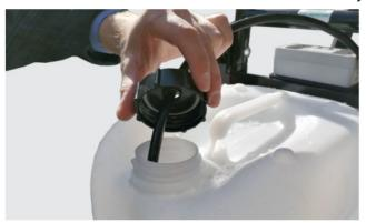
4. Insert your telescopic pole hose directly to the water outlet connection (it is possible to add a 100mtr hose reel in between your STREAMFLO® system and the telescopic pole).
