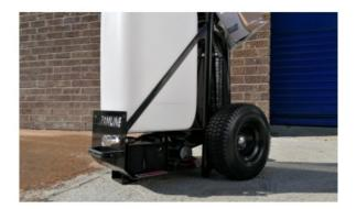
2. Remove the container lids and riser tube and fill the container with pre-filtered water. If the trolley is fitted with a resin filter fill the container with tap water.
