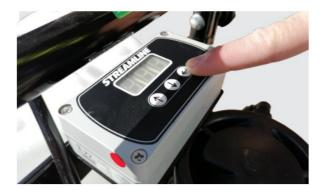
2. Now you can adjust the speed of the water flow through the 100psi pump by using the and arrows on the flow controller.
