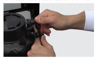
3. Unscrew the filter bracket and remove the DI filter from the trolley.
