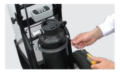
4. Remove the DI filter head and empty the poor/spent DI resin.
