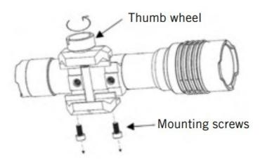
Align the M-LOK® mount holes with the ProTac 2.0 Rail Mount holes and use the 3/32'' hex wrench to tighten the  $8-32\times1/4''$  screws.
