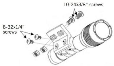
To connect the ProTac 2.0 Rail Mount and M-LOK® mount to the rail, rotate the M-LOK® T-nuts to the install/uninstall position. Position this assembly in the desired rail location. Tighten the 10-24×3/8" screws using the 1/8" hex wrench to lock the T-nut.
