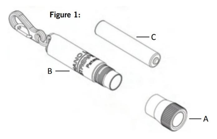
Use a single AAAA alkaline battery. To change, remove head (A) and old battery (C). Install a fresh battery, with negative end into the barrel (B). Replace the head (A). If the LED doesn't light, confirm that the battery has the correct orientation.
