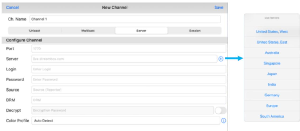
The screenshot shows the 'New Channel' configuration window with 'Server' mode selected. The 'Server' field contains 'live.streambox.com'. A blue arrow points from the dropdown icon next to the 'Server' field to a 'Live Servers' pop-out menu. The pop-out menu lists the following server locations: United States, West; United States, East; Australia; Singapore; Japan; India; Germany; Europe; and South America.
