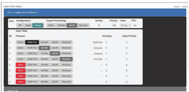
Each Output port of the Gateway also has a VisionNet Confi guration similar to the VN to DMX Interface card. These confi gurations can be assigned output ports with or without DMX Module representing them. Populating this from the designer requires selecting the Gateway VN Interface option for outputs, and the appropriate Gateway Port and Gateway ID:
