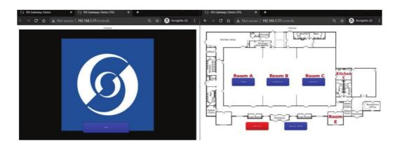
Example – with a Vision.Net confi guration in a building with multiple ballrooms: an OTG screen could be confi guard such that one Gateway would allow the people using each ballroom/conference room to access and control their areas simultaneously without interfering with the other rooms.
