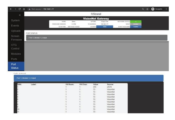
This tab is required Admin Level access, a DMX Module attached to the Gateway, RDM on the Modules tab to be set to On, and one of the DMX Module's ports being confi figured as an output. Without this setup, the RDM tab is not functional:
