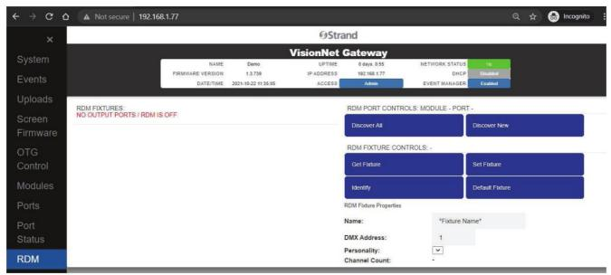
If the Confi guration matches up correctly, then the web page allows for basic Port level RDM Discovery and Fixture Confi guration (Fixture name, DMX Address, Personality, Identify, Default Fixture...):
