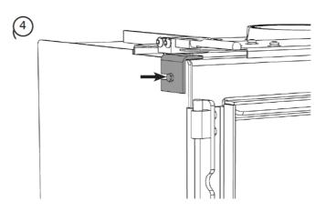
When installed the bracket locates on the top left of the inner box.
