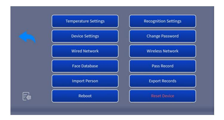
**Temperature Settings:** Click the temperature unit option to switch between Celsius and Fahrenheit; the warning value is the high temperature threshold.
