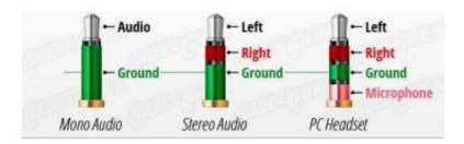
Notes: Application software should always ensure the same audio is present on both Left and Right Channels for correct mono operation. Headsets with microphones can be used but there is no microphone support.
