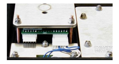
• P1 is the input connector for the buttons (6-way) and is always fitted.
