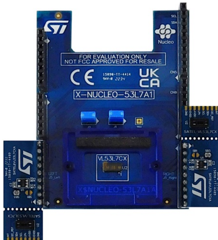
Figure 6. SATEL-VL53L7CX breakout boards connected to the X-NUCLEO-53L7A1 expansion board
