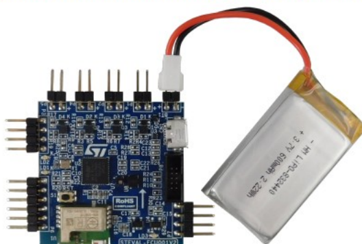
Figure 15. STEVAL-FCU001V2 and LiPo battery connection
