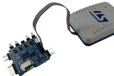
Figure 7. ST-LINK/V3 connected to the STEVAL-FCU001V2 evaluation board via adapter
