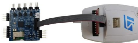
Figure 7. ST-LINK/V3 connected to the STEVAL-FCU001V2 evaluation board via adapter
