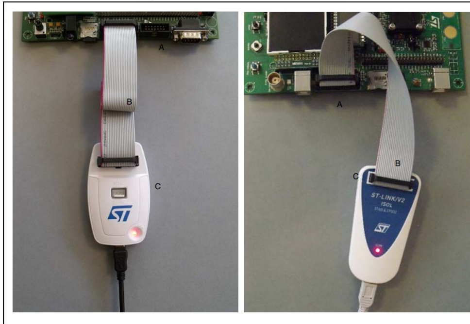
Figure 9. JTAG and SWD connection
