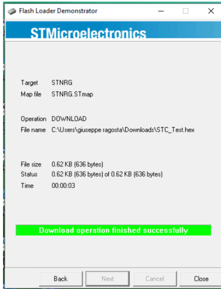
Figure 10. ST Flash Loader – STNRG programming complete
