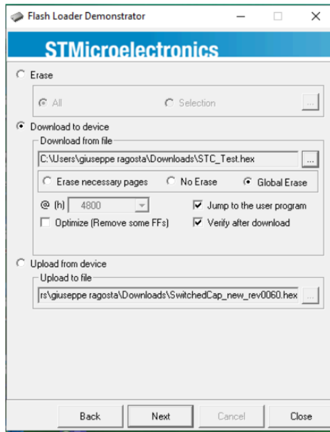
Figure 9. ST Flash Loader – STNRG programming settings
